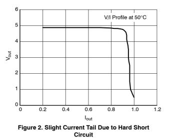
For output of 12 or 15 volts this may cause a more prominent current tail which may not necessarily pass a hard short circuit condition.
